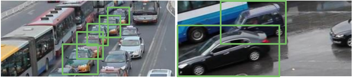
Fig. 6.7: Partial occlusion in the UA-DETRAC dataset where the object BBOX covers a great part of the region belonging to another object.
