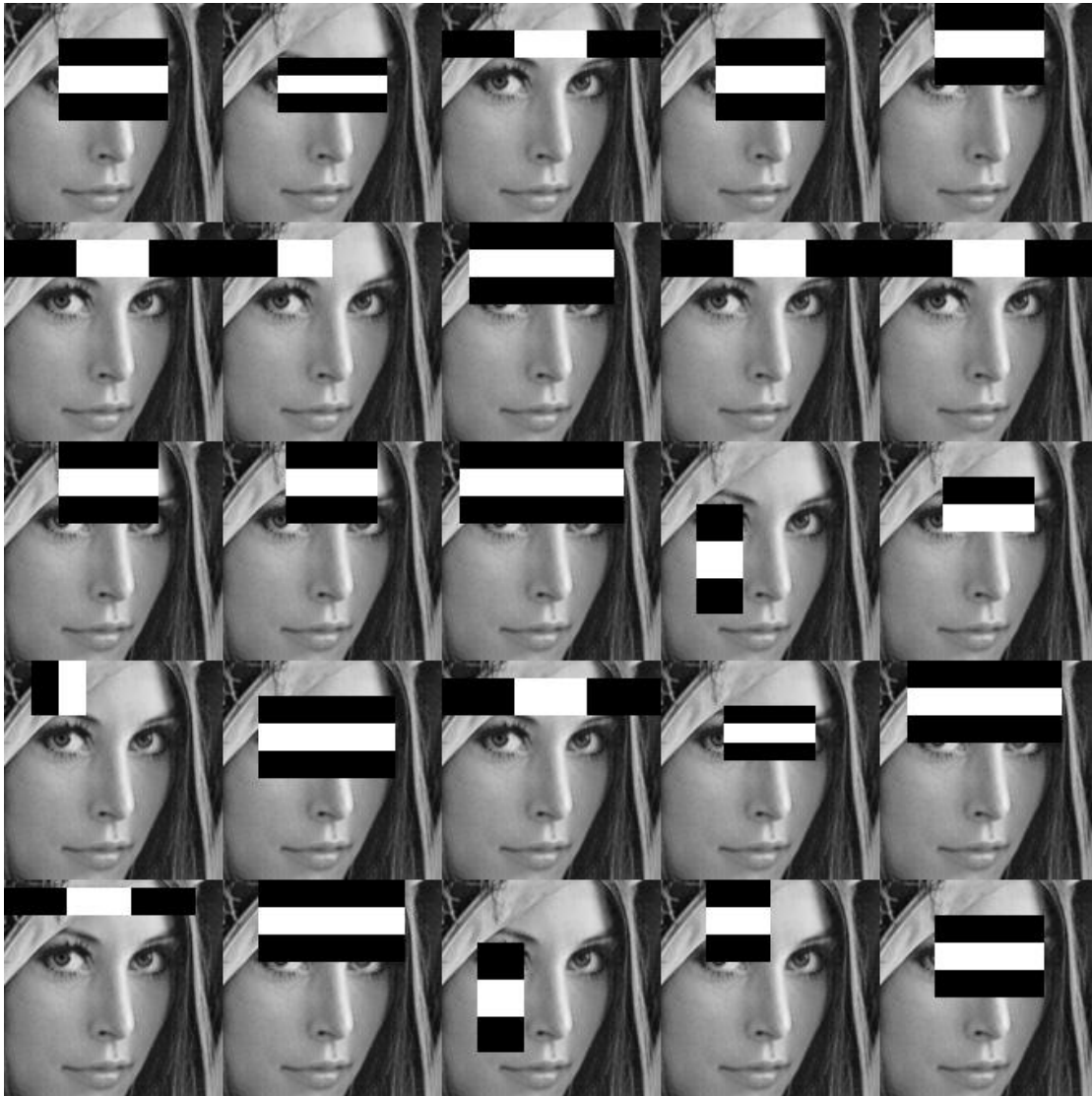
Figure 3: Example of Haar Wavelets. The rectangles represent a specific Haar Wavelet. The squares are summed up, with black taken as negative and white as positive values, producing one feature.
